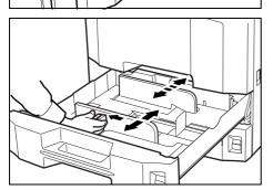
2 Holding the paper width adjusting tab, move the paper width guides to fit the paper.
